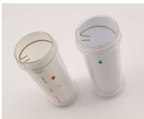
Fig. 1. Test tubes. Left: a holding tube (green dot) with a steel clip (ring) and an exposure tube (red dot) with a copper clip. Right: a holding tube (green dot) connected to an exposure tube (red dot) with a slide unit
