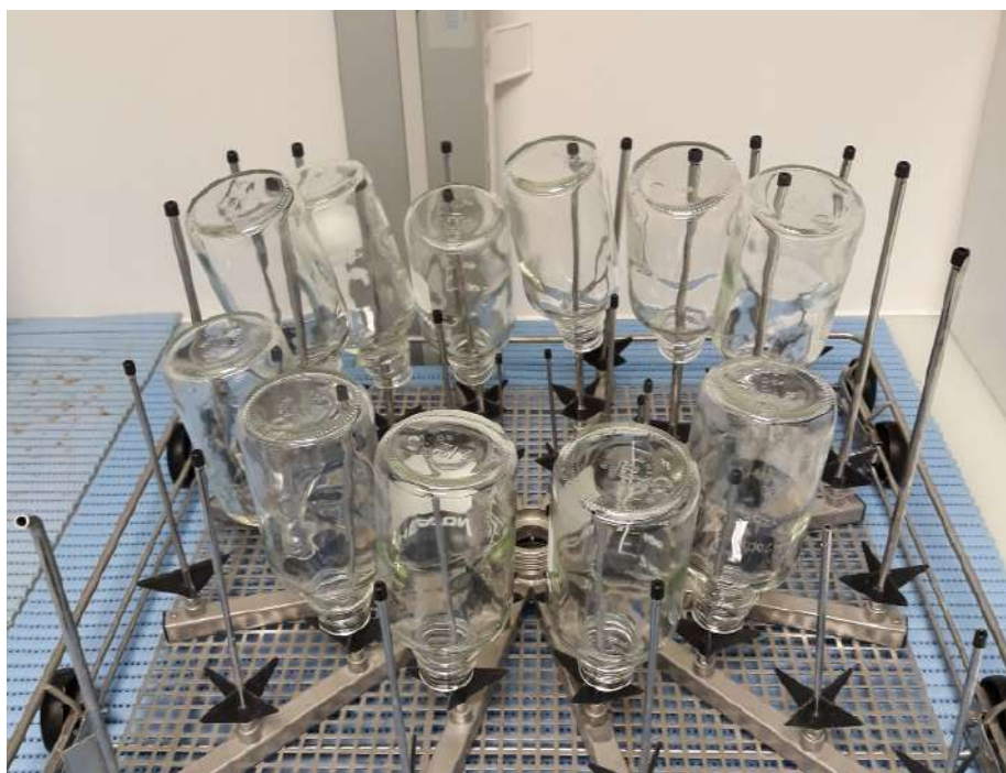
Fig. 4. Method of drying glass bottles upside down on raised steel rods
