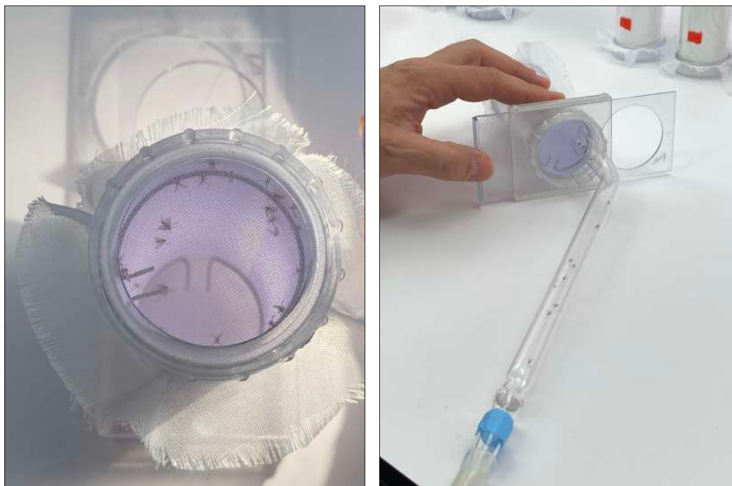
Fig 2. Netting screen on bioassay tubes (hole size, < 500 µm) that prevents escape of sand flies during testing (left); introducing sand flies into the tube (right) (photo credit: IRD/Dr Stéphane Duchon)
