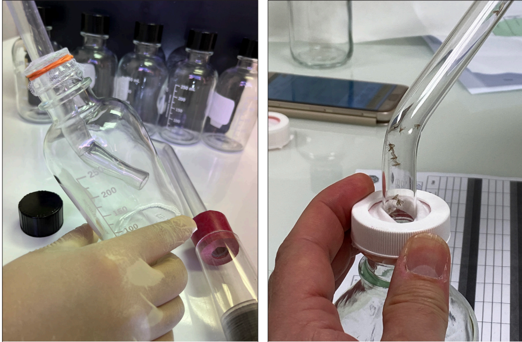
Fig 3. Showing technique for introduction of sand flies into a 250-mL glass bottle a with a holed netting piece (left) (photo credit: WHO/Dr Rajpal Yadav); a glass bottle with a holed cap and a rubber flap for introduction of sand flies as an alternative technique (right) (photo credit: IRD/Dr Stéphane Duchon)
