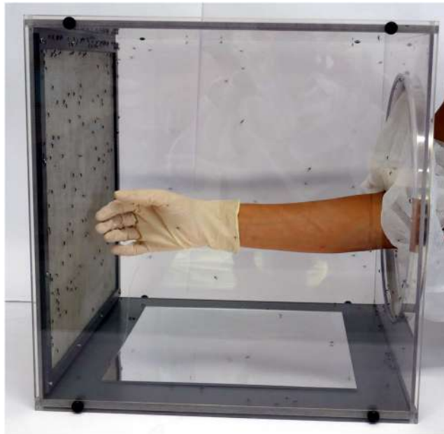
Figure 2. The arm-in-cage (AIC) test for measuring the efficacy of topical mosquito repellents under laboratory conditions. Hungry female mosquitoes are contained in a test cage and the repellent is applied to the forearm between the wrist and elbow, while the hand is protected by a latex glove through which the mosquitoes cannot bite.
